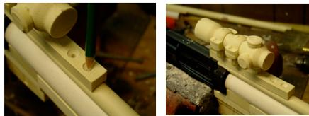
Screw the scope rail on, and glue it down as well, this will help keep it aligned even. While the glue is drying, you will need to cut the tip of the barrel off your airsoft gun.
