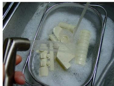
It is very important to wash your resin parts in very warm soapy water, then rinse well and allowed to dry. A mold release agent was used and has to be removed prior to paint-
