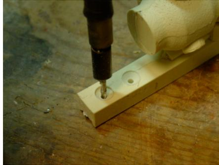
The scope base needs two holes drilled and counter sunk.
