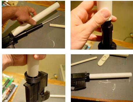
assemble the parts. We started with the barrel pipe. The shorter of the two 1/2 diameter pipes. Add the pipe adaptor and the end cap. Super glue them on.
