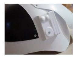
The com box needs special attention when trimming to ensure a good fit. Guidelines have been marked in pencil, but take it easy. Trim a small amount and test fit. Go slow.
