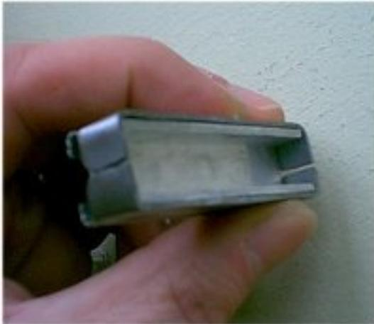
Cut a section the same length as the clamp tube. Next cut two pieces of steel which will stick to the sides of this and wrap around the ends so that they touch each other in the middle of the two ends. To get them to wrap neatly file slots with the triangular needle file on the inside where you want to bend them, this will make the bends near 90 degrees rather than a curve.
