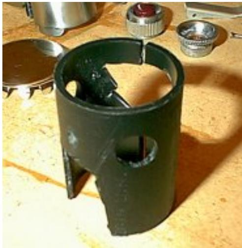
Now take the black waste tube and cut a section then cut down the side so it can be opened up (as it's not quite wide enough - but we'll solve that). Drill a hole for the screw above the eye and the two recharge sockets, leave it little higher than the edge of the tube to give the correct look. You will need to use a craft knife to trim the edges of the cuts as they are left ragged by the drill. Now is a good time to cut out the sections for the other holes as well.
