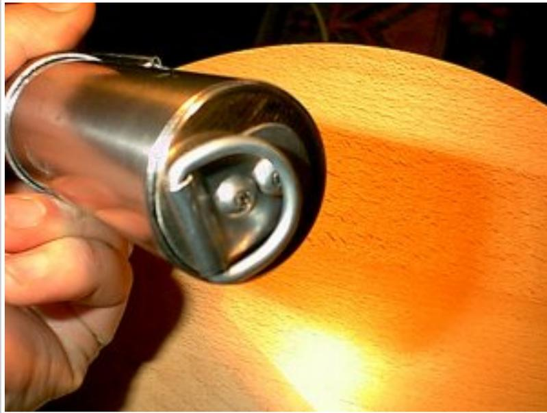
Take a strip of steel and bend a right angle in it, now wrap it around the D-ring, round off the end and drill two holes through this tab and the end plug. Screw them onto the end plug. Glue this in place in the bottom of the tube.
