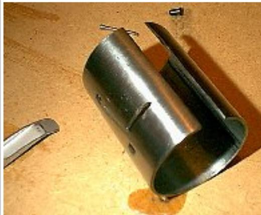
Firstly, lets get the clamp band onto the main tube. You can use the [plan](#) to estimate where the band goes (I put the bottom edge 90mm from the base of the main tube), put some grease on the inside as we will use a screw to keep it in place like the original. Once it's in the right place mark and drill a hole for the the clamp band screw the right size to screw into securely (I did all this with the band in place).
