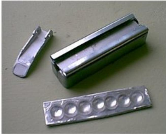
The clamp is very easy to make compared to most of the other parts, the main reason being that it is based on a short section of aluminium square "U" section rod.
