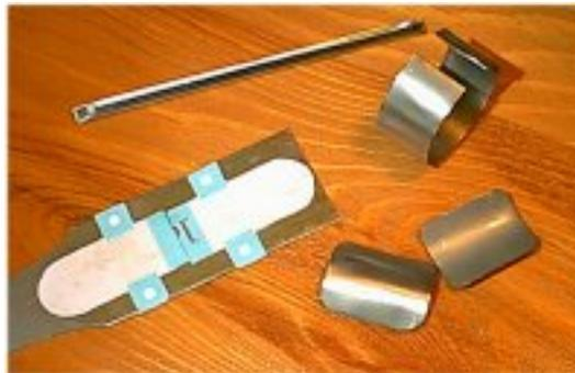
Cut a strip of steel the same width as the Reflex template but a little longer. Now wrap this around a cylinder (look around the house for something approximating the diameter, the bathroom is a good bet) to get a clean cylinder shape.
